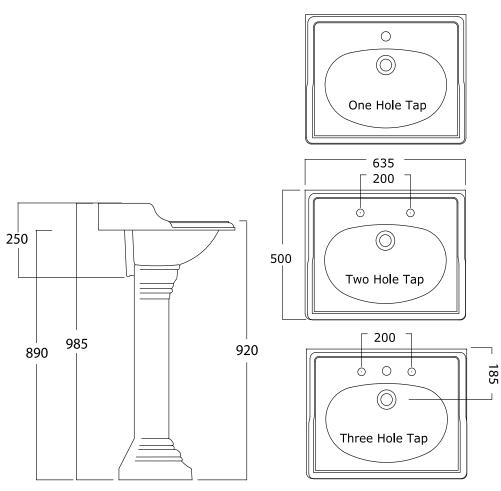
Open cavity at back of pedestal to the floor for floor outlet
