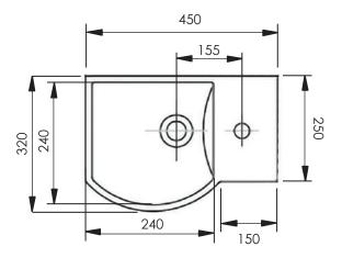
DIAGRAMS NOT TO SCALE | ALL DIMENSIONS IN MM TOLERANCE OF  $\pm$  5MM  $\,$  ALL PRODUCTS CONFORM TO BRITISH STANDARDS  $\,$
